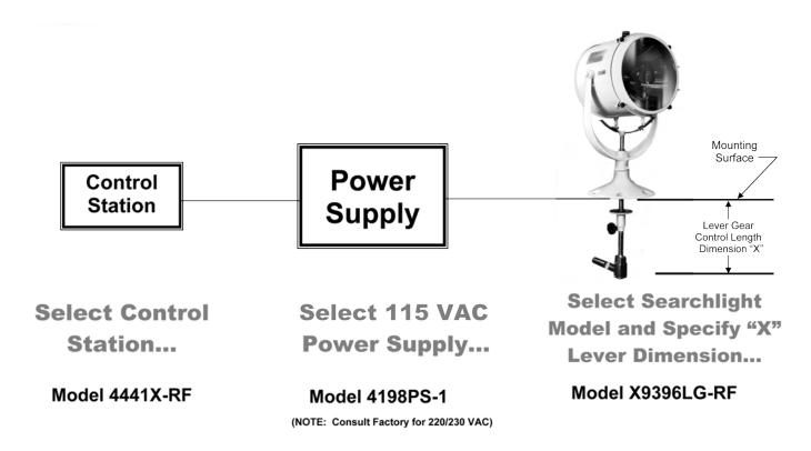
**How to Specify...** Each system consists of (1) Searchlight Model X9396LG-RF, (1) 115 VAC Power Supply Model Number 4198PS-1 and (1) Control Station Model 4441X-RF. The lever gear control length, i.e. Dimension "X", is a standard length of 22-inches. Customer can specify a custom dimension, by providing
